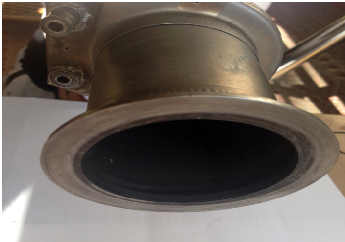
Figure 1: Air supply ducting of a B737 aircraft [35].
