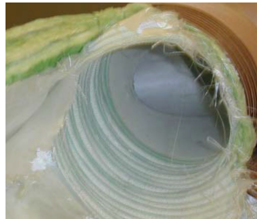
Figure 3: Unused air supply ducting [7].
