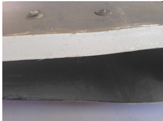
Figure 2: Turbo compressor ducting of a non-bleed air aircraft, Vickers VC 10 [35].
