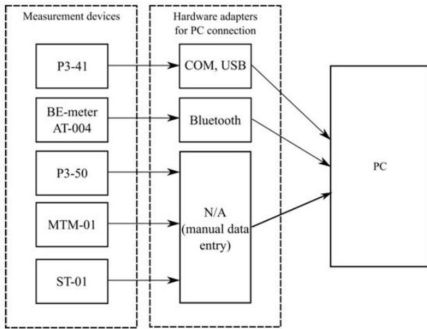
Figure 1: Connection of measurement devices to PC.
