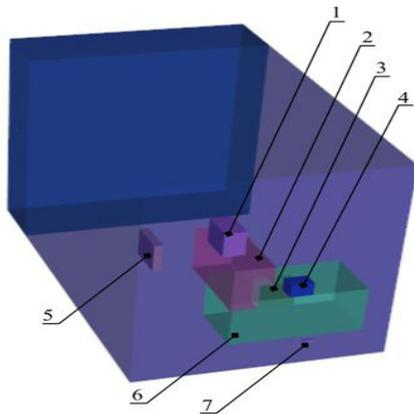
**Figure 5:** 3D Model of a Studied Room with Electromagnetic Field Sources: 1 - LCD Display, 2 - Table, 3 - PC System Block, 4 - Notebook, 5 - Electric Heating Device, 6 - Table, 7 - Notebook Power Adapter.
