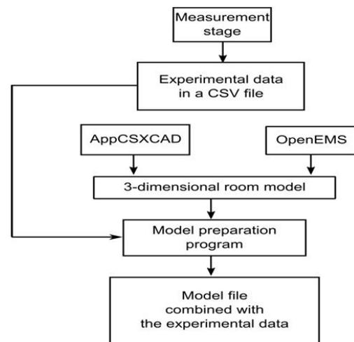
Figure 4: Experimental Data Processing Diagram.
