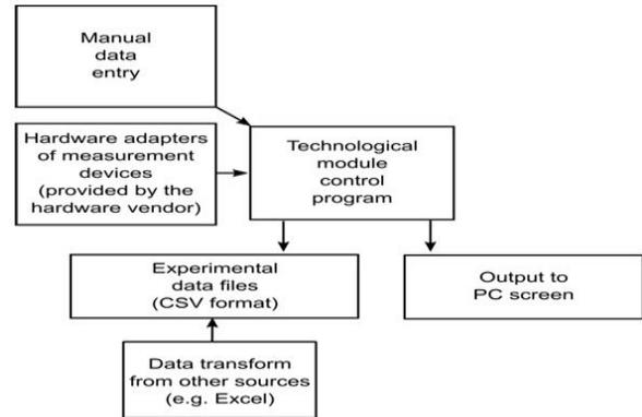
Figure 3: Experimental Data Flow Diagram.
