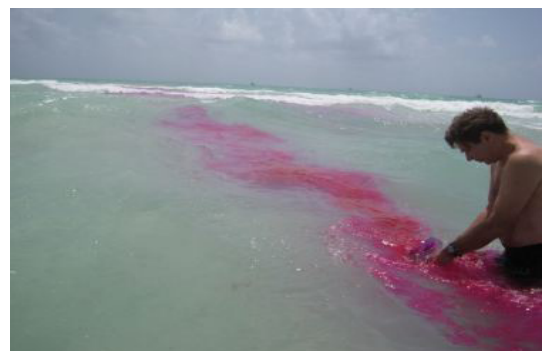
Figure 2: A clear-water rip current at Miami Beach, Florida as delineated by red fluorescent tracer dye.
