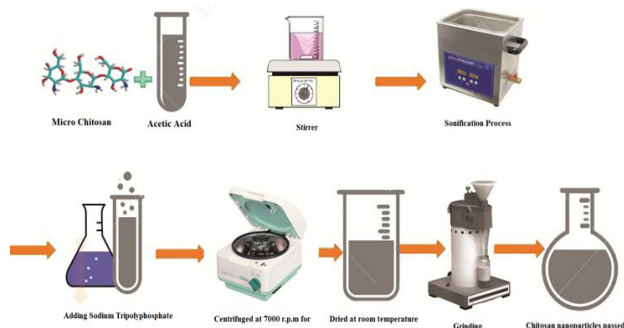
Figure 1: Schematic Diagram of Producing Chitosan Nano Particles Via Method of Chemical Hydrolysis.
